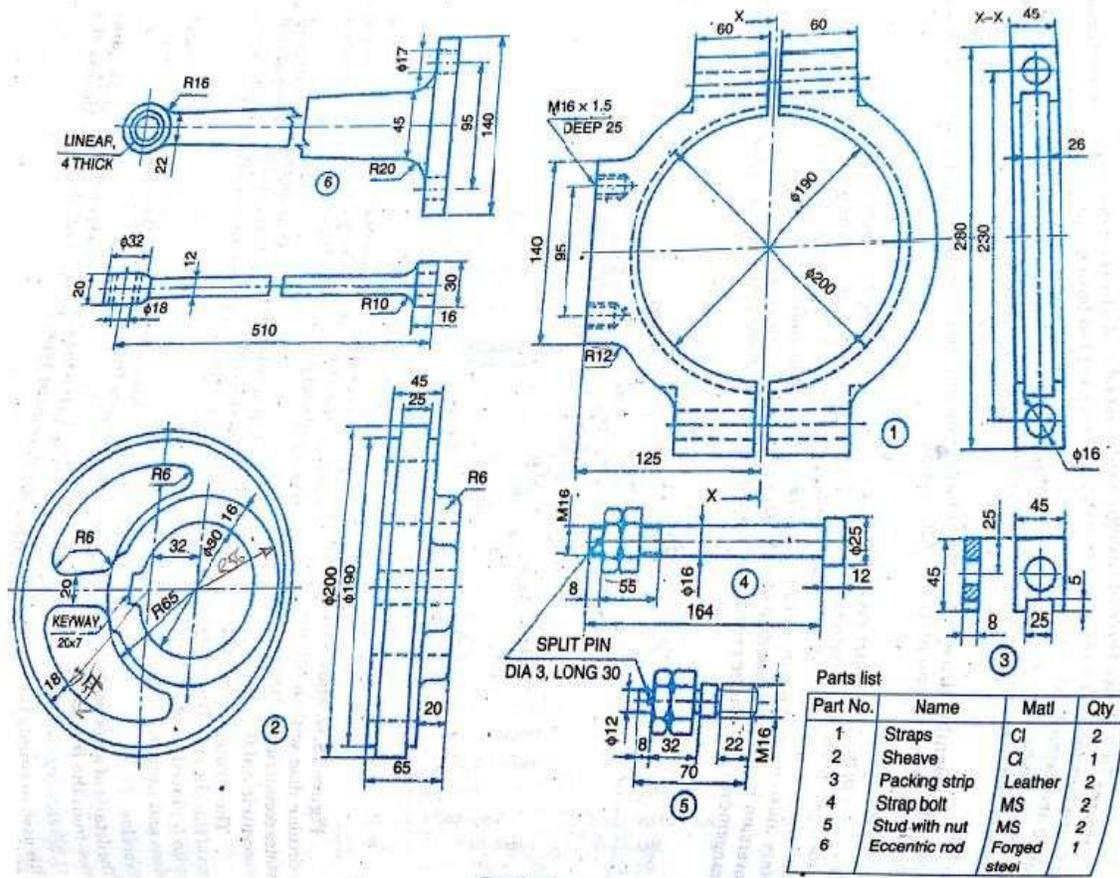
Fig:Details of an Eccentric
