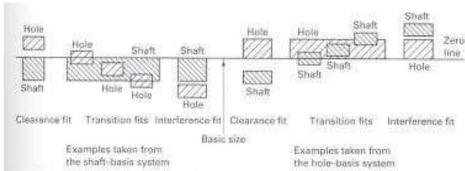
Hole basis and shaft basis system
