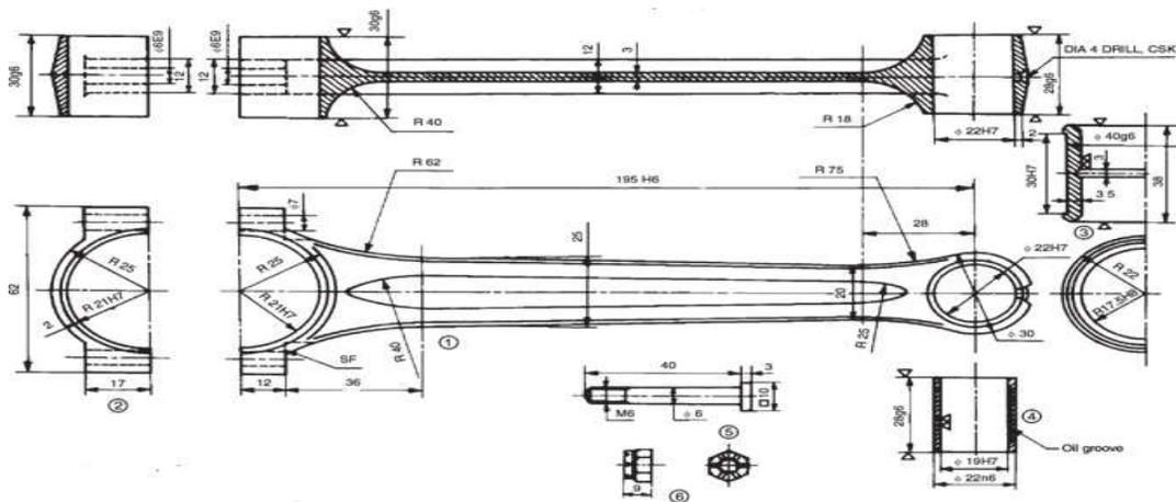
Fig. Details of a Petrol engine connecting rod
